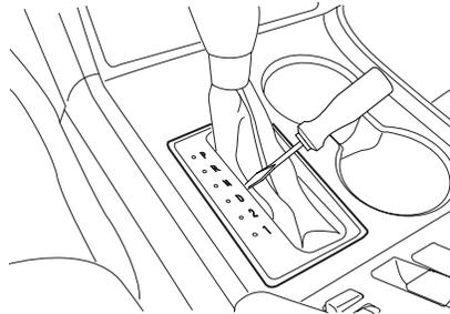
3. Pull the bezel assembly up far enough to expose the inside of the gearshift lever compartment.
