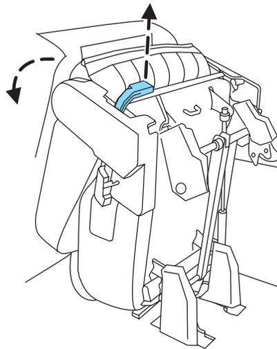
2. Pull up on the handle located at the back of the seat. The seat will flip forward.
