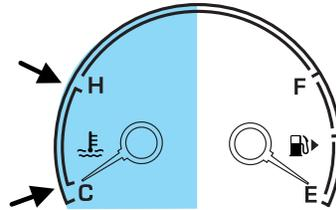
If the engine reaches a preset over-temperature condition, the engine will automatically switch to alternating cylinder operation. Each disabled cylinder acts as an air pump and cools the engine.
