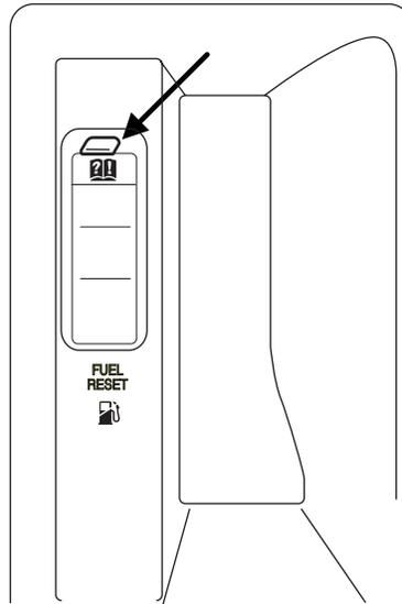
The fuel pump shut-off switch has a red reset button on top of it and is located beneath the air suspension switch (if equipped). If the vehicle is not equipped with air suspension, the fuel pump shut-off switch's red reset button will still be visible behind this access panel.
