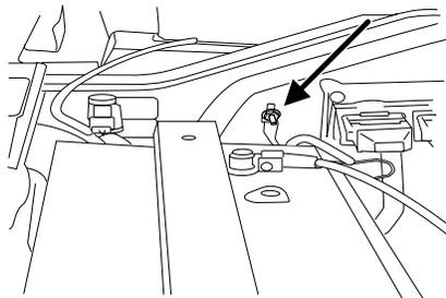
4. Make the final connection of the negative (-) cable to the jump starting stud located in the rear of the engine compartment, near the battery. **Do not** use fuel lines, engine rocker covers or the intake manifold as *grounding* points.
