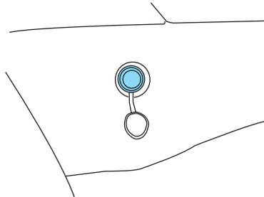
A second auxiliary power point is located inside the cupholder door on the rear side of the center console. The power point is accessible from the rear seats.
