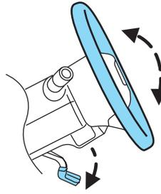
While holding the steering wheel, pull the lever up to its original position to lock the steering column.
