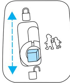
Move lock control up to engage the childproof lock. Move control down to disengage childproof locks.
