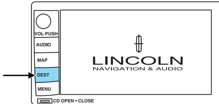
Press DEST on the main bezel to access the navigation mode.
