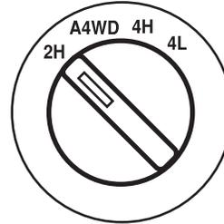
**Note:** If your vehicle is equipped with AdvanceTrac<sup>™</sup>, the AdvanceTrac<sup>™</sup> system will automatically turn off the stability enhancement feature when you shift the Control Trac A4WD system into 4L (4X4 LOW). The brake traction enhancement feature will still be enabled.
