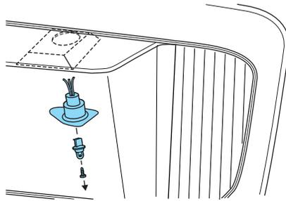
5. Install the bulb socket in the lamp assembly by turning it clockwise.
