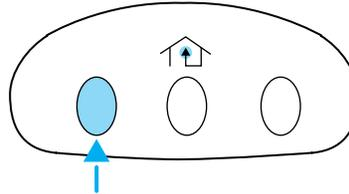
4. The red light will flash slowly and then rapidly. Release both buttons when the red light flashes rapidly. (The rapid flashing light indicates acceptance of the hand-held transmitters' radio frequency signals.)
