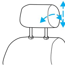
Push control to lower head restraint.
