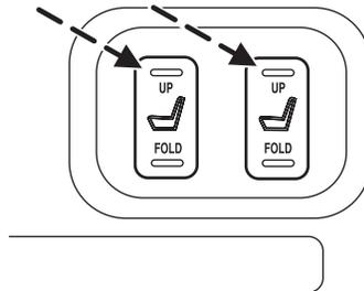
**The power folding seats are designed to stall within 1–10 seconds of encountering an obstruction when opening or closing. Should this occur, remove the obstruction and wait approximately 1–4 minutes for the seat motor to reset.**
