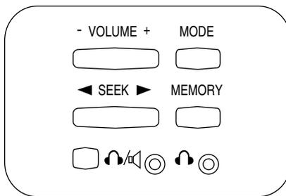
When the rear seat controls are activated, rear seat passengers can use the controls to change the playing media for all passengers (Single Play mode). In this mode, all speakers will play audio from the same media source for all passengers to hear. To activate the rear seat radio controls:
