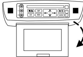
The screen rotates down to view and into the housing to store when not in use. Be sure the screen is latched into the housing when being stored.
