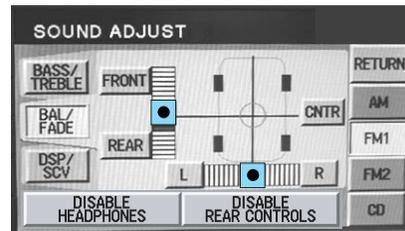
**SCV** (Speed Compensated Volume) Automatically compensates for road wind and noise. Refer to *Speed compensated volume* earlier in this chapter.
