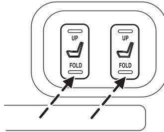
Push the top of the control button to return the seatback to its original position.
