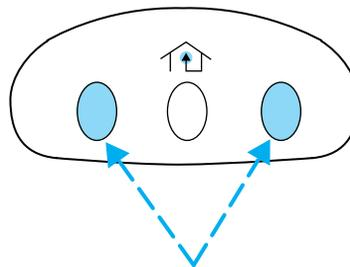
2. Position the end of your hand-held transmitter 2–8 cm (1–3 inches) away from the HomeLink® Universal Transceiver surface (located on your visor) while keeping the red light in view.
