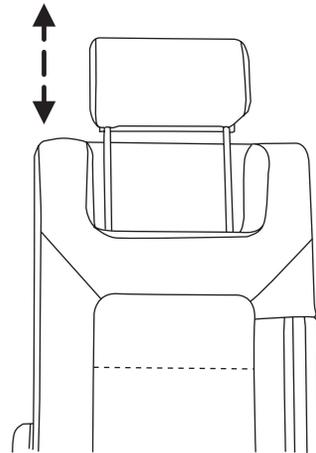
Push control to lower head restraint.
