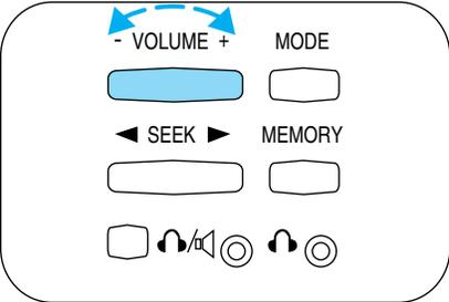
From the rear seat controls, volume control can be set no higher than the current radio setting unless the speakers are turned off.
