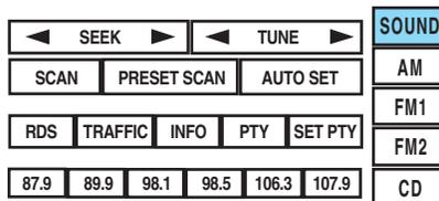
The AM/FM control works in radio, CD and navigation modes.
