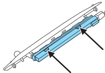
5. Pull the old bulb out and replace with the new bulb.
