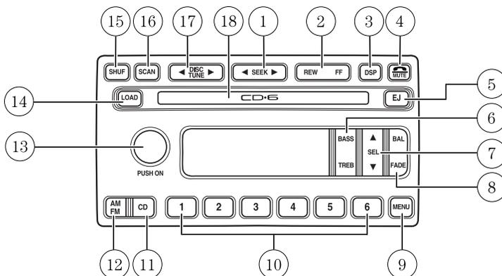
1. **SEEK:** Works in radio or CD mode. Press and release SEEK ◀ / ▶ for previous/next strong station, or track of current disc.
