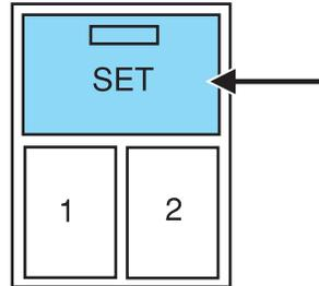
A position can only be recalled when the transmission gearshift is in Park. A memory position may be programmed at any time.
