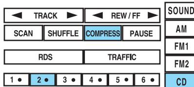
When in CD or CDDJ mode, press COMPRESS to engage or disengage the compression feature.
