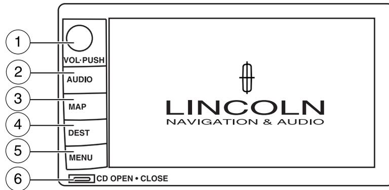
1. **VOL-PUSH:** Press to turn the system ON/OFF. Turn to adjust the audio volume level.
