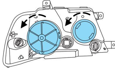
6. Once the bulb covers are removed, the bulbs can be removed by turning them counterclockwise and then pulling the bulbs straight out.
