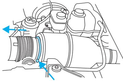
2. Loosen the clamp that secures the air filter cover to the air filter housing and carefully separate the cover from housing.
