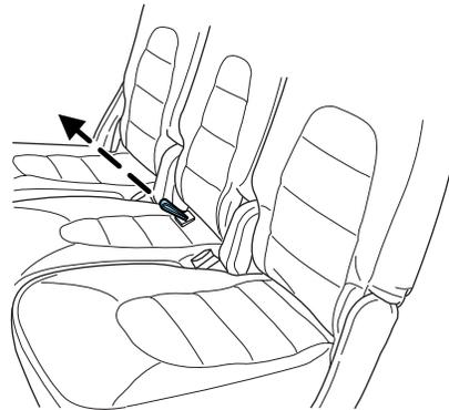
2. With the latch released the seatback can be lowered into the load floor position.
