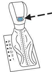
When you shut off and re-start your vehicle, the transmission will automatically return to normal **D** (Overdrive) mode.
