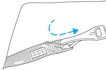
6. Tighten the child safety seat tether strap according to the manufacturer's instructions.
