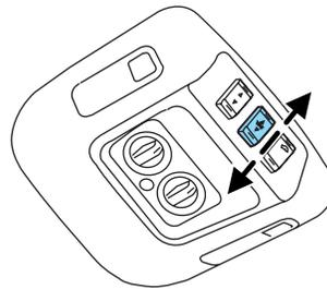
Press the ▲ portion of the VENT control to open the power rear quarter windows.
