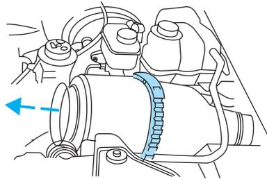
3. Remove the air filter element from the air filter housing.
