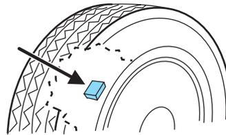
**must be unbolted from the wheel prior to tire removal. The sensor can be removed by loosening the nut at the valve stem. Failure to remove the sensor may damage it.** The rubber grommet (washer) between the wheel and the tire pressure sensor needs to be replaced when any tire is changed to minimize air leaks.
