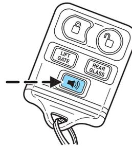
To deactivate the alarm, press the control again or turn the ignition to ACC or ON.
