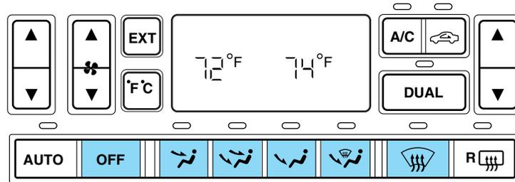
The manual override controls allow you to determine where airflow is directed. To return to full automatic control, press AUTO.
