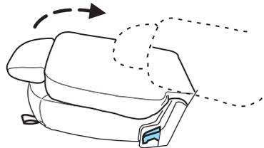
2. With the seat in the flat back position, lift up on the lever located on the side of the seat cushion. This will allow the seat back to be lifted to the upright locked position.
