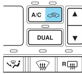
The recirculated air cannot be selected in Defrost, as interior fogging may occur. To reduce the risk of fogging while in Floor & Defrost, the recirculated air can be enabled for approximately 4 minutes and the recirculated air indicator will be lit. After approximately 4 minutes of recirculated air operation while in Floor & Defrost, the DEATC (Dual Electronic Automatic Temperature Control) will automatically disable the recirculation control and the recirculated air indicator will not be lit.
