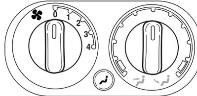
The auxiliary climate control system is dependent on the main climate control system. If the main climate control system is in the Off position, the auxiliary climate control will not operate. If the main climate control system is on, the auxiliary air will not be cooled unless the air conditioning is functioning on the main climate control system.
