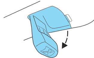
The conversation mirror on the cover allows the driver to view the rear seating area.
