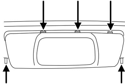
3. Hold the cover against the bumper trim and reinstall the two screws.
