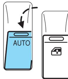
If the switch is pressed and held to the normal close or ONE TOUCH UP position during a ONE TOUCH DOWN event, the window will stop. If, after 1/2 second the switch is still held, the window will perform a normal close or ONE TOUCH UP.
