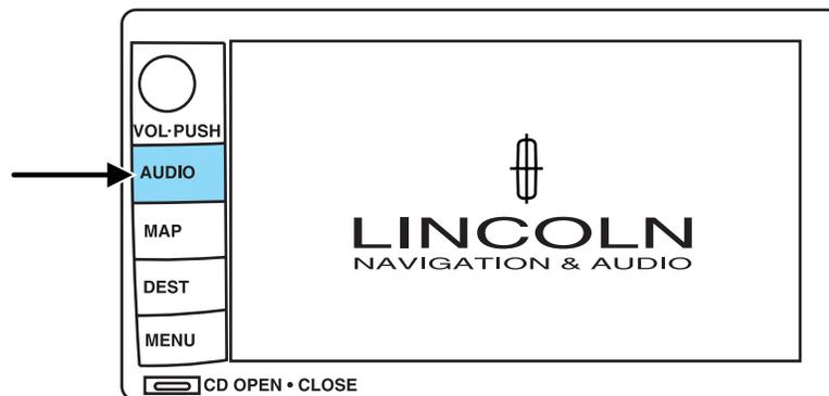
Your Lincoln Navigation Audio System has many features including a full range of audio functions. To access these functions, press AUDIO on the main bezel. This will take you into audio mode.
